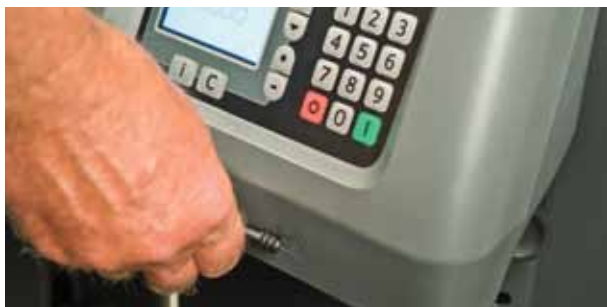
BT Optio H-series requires either a PIN-code or an ID key (option) to start
