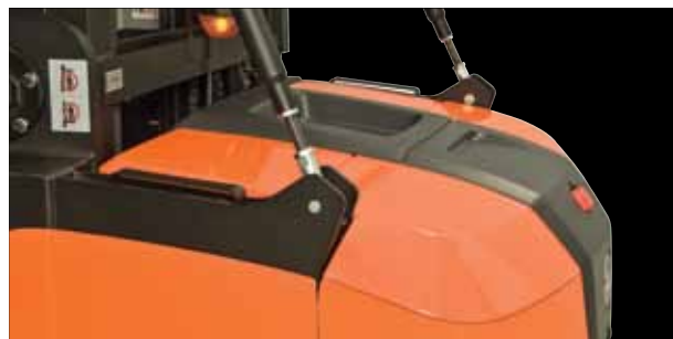
Non-exposed parts, such as the battery cover, are made of plastic to save weight
