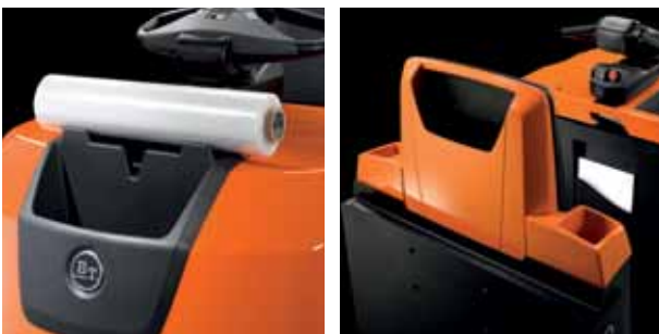
BT Optio L-series offers useful front and rear storage compartments. The front compartment even has a rest for shrink wrap
