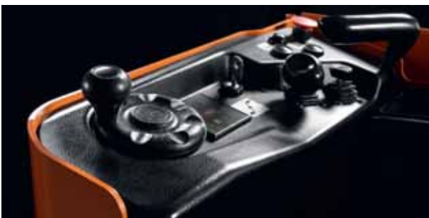
The LSE200's 180° steering makes it easy to drive
