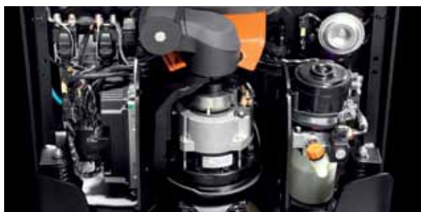
The fixed motor has no moving cables
