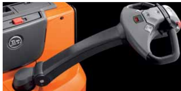
The control arm incorporates BT Powerdrive technology and offers easy, intuitive operation
