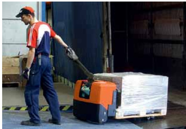
The LWE130 is well suited for use on a lorry and for handling loads on a rear mounted lorry platform
